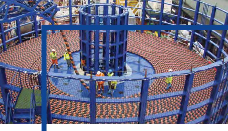
At the cable factory in Cologne, submarine cables weighing many tonnes can be stored on a turntable before shipment to customers
